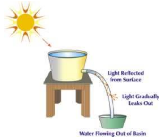
Figure 1 - John Tyndall's Experiment
