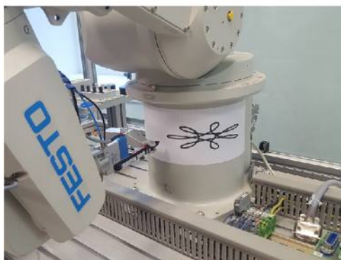
A hypotrochoid drawn by the robot on the a curved (cylindrical) surface
