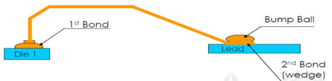
Figure 2 : Bond Ball On Stitch (BBOS)
