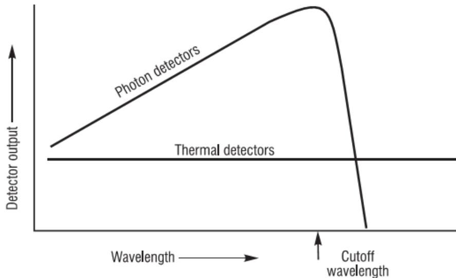
Figure 5.1 – Schematic drawing of the relative output per unit input for photon detectors and thermal detectors as a function of wavelength. The position of the long-wavelength cutoff for photon detectors is indicated [11]
