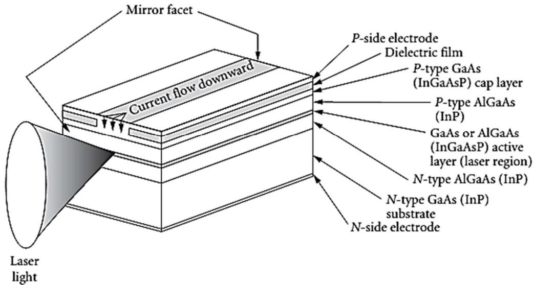
Figure4.13 – A typical heterostructure semiconductor laser showing various layers of differential materials and the narrow region, where current flows to produce the gain region in the active layer [1]
