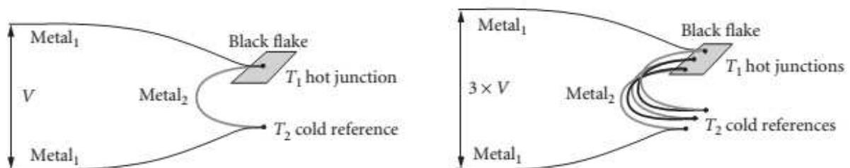
Figure 7.1 – a) Thermocouple detector structure; b) Thermopile detector structure [1]
