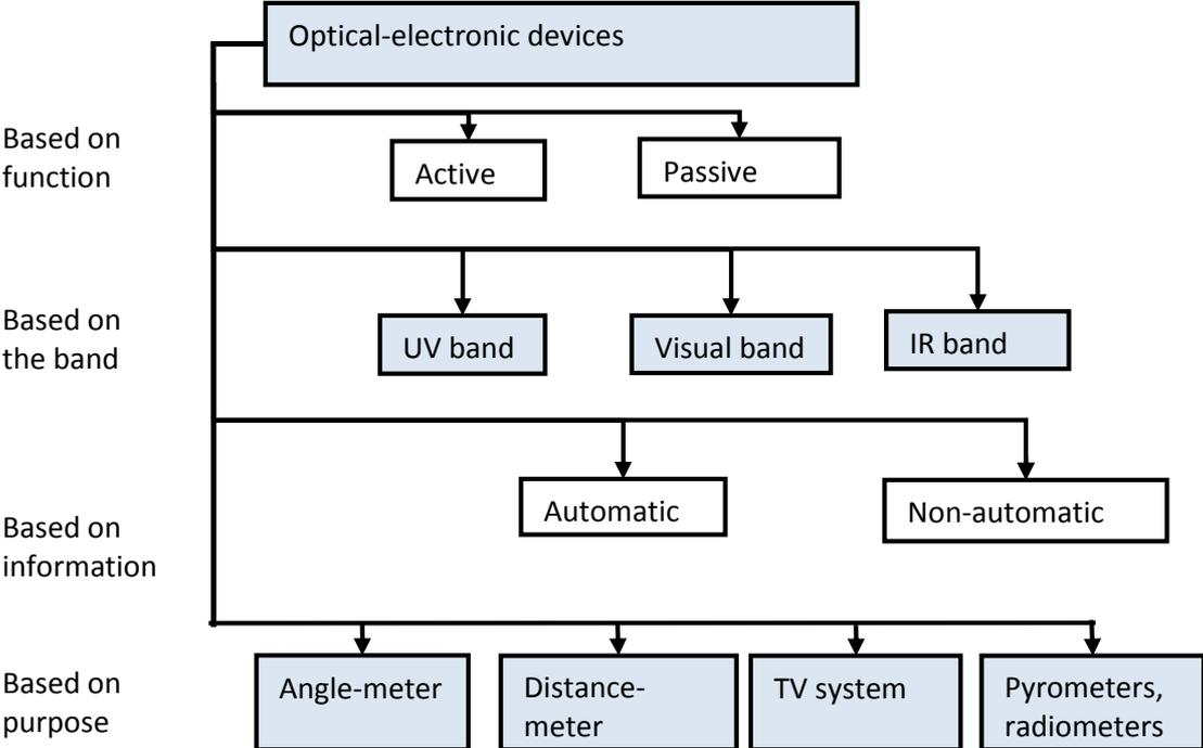
Figure 1.2 – Classification of optical-electronic systems
