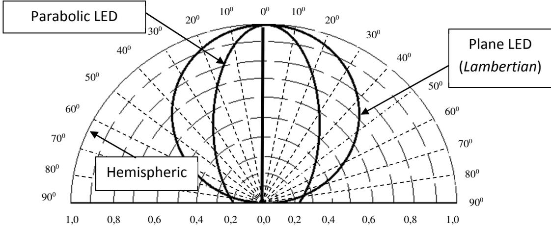
Figure4.7 – Light diagram of LEDs for various package types
