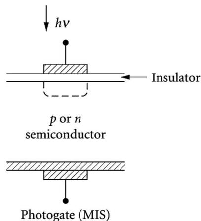
Figure 8.1 – Metal-insulator-semiconductor structure
