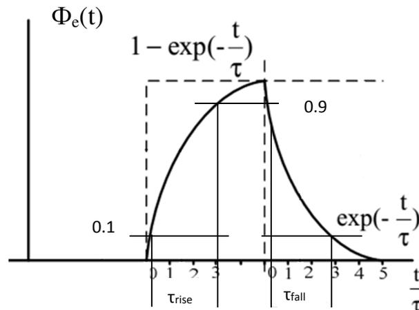
Figure 5.4 – Detector rise and fall times
