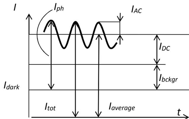
Figure 5.2 — Structure of the total detector current
