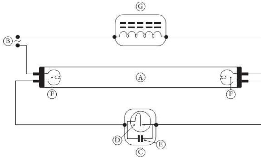
Figure 4.4 – A preheat fluorescent lamp circuit using an automatic starting switch. A—fluorescent tube with fill gases, B—power, C—starter, D—switch (bimetallic thermostat), E—capacitor, F—filaments, and G—ballast
