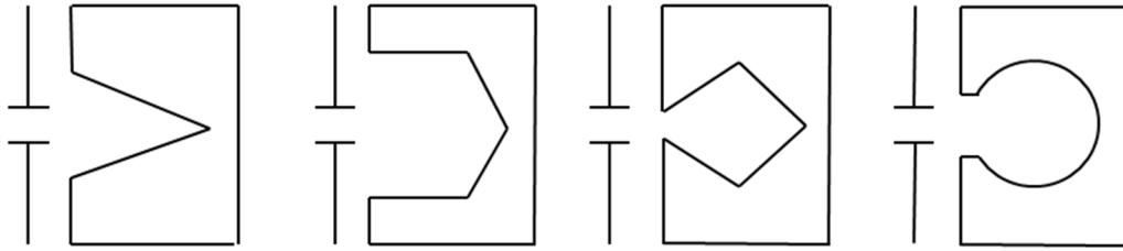
Figure 4.1 — Cavities of a blackbody model
