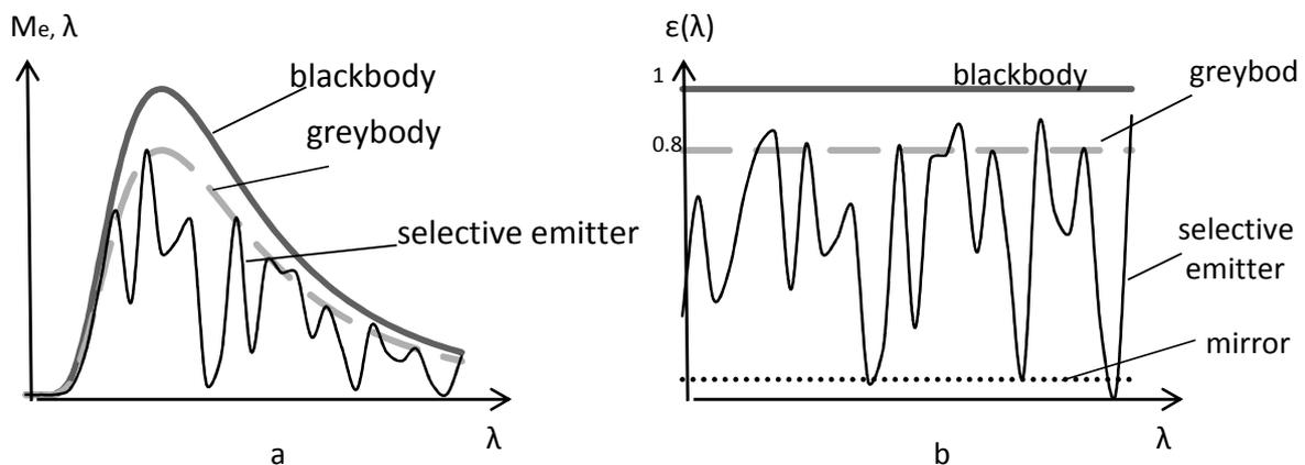
Figure 3.3 – (a) Radiant emittance spectral density for different emitter types; (b) emittance vs wavelength diagram for different emitter types
