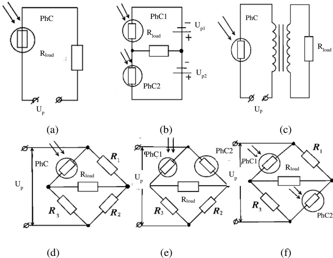
Figure 6.4 –Recommended circuits for photoconductors
