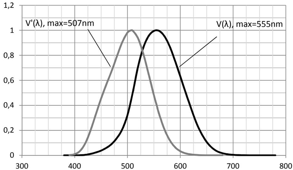
Figure 2.5 — CIE  $V(\lambda)$  and  $V'(\lambda)$  functions
