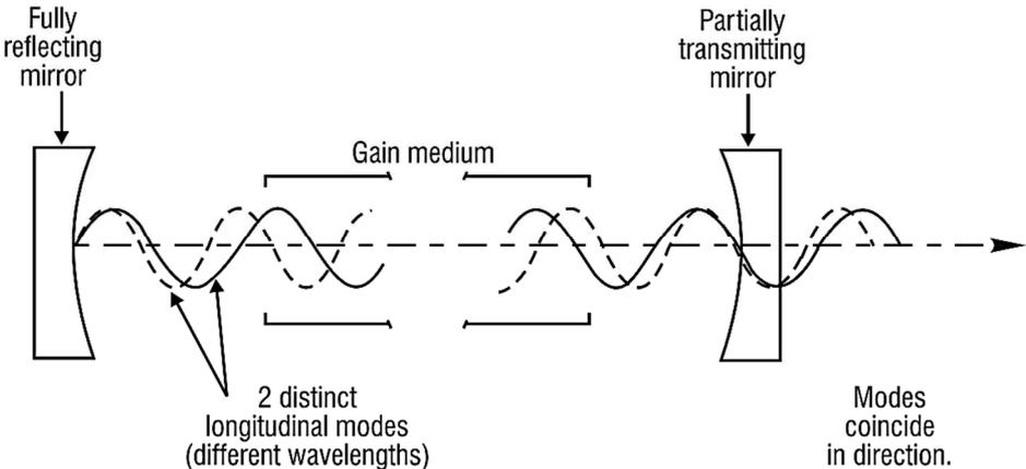
Figure 4.11 – Two distinct longitudinal modes operating simultaneously in the same laser cavity
