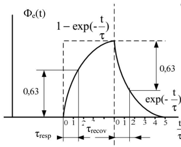
Figure 5.3 – Detector response and recovery times
