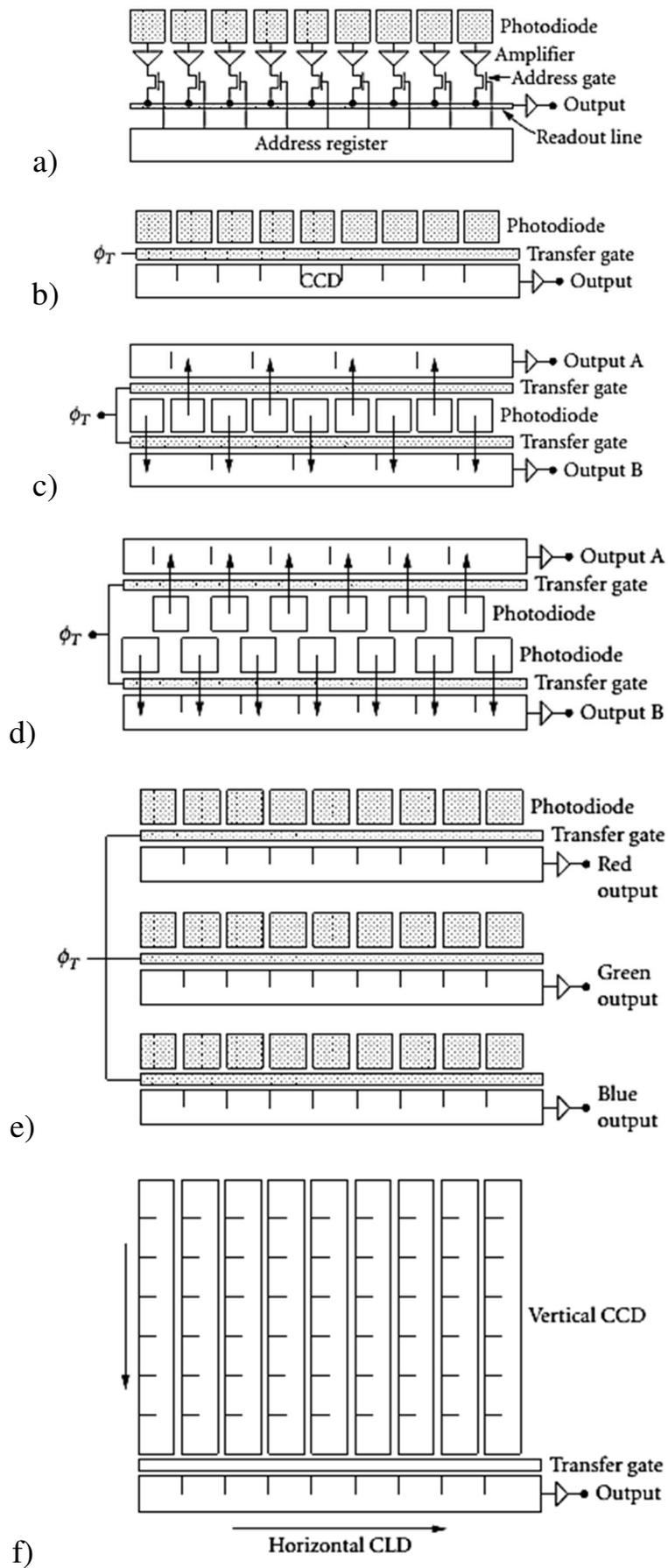
Figure 8.3 — Architectures for linear image sensors
