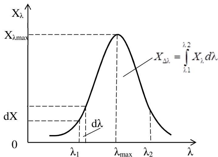
Figure 2.4 – Spectral density distribution of a photometric quantity  $X_\lambda(\lambda)$
