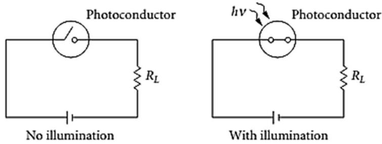
Figure 6.3 –Equivalent circuit diagram of a photoconductor
