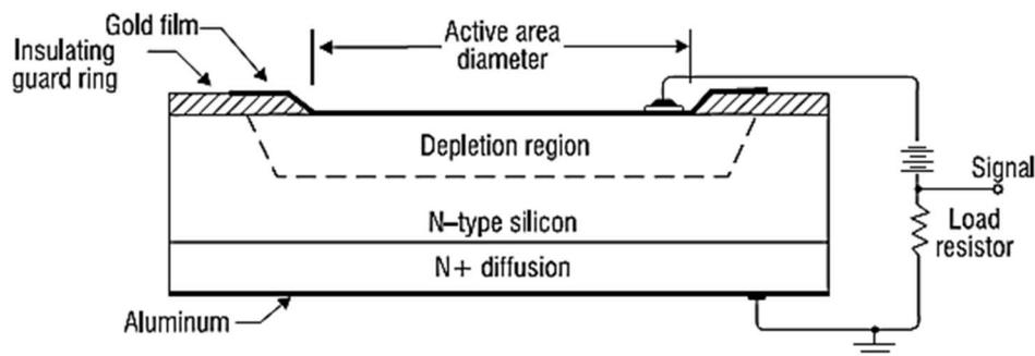
Figure 6.11 — Schottky photodiode structure [11]
