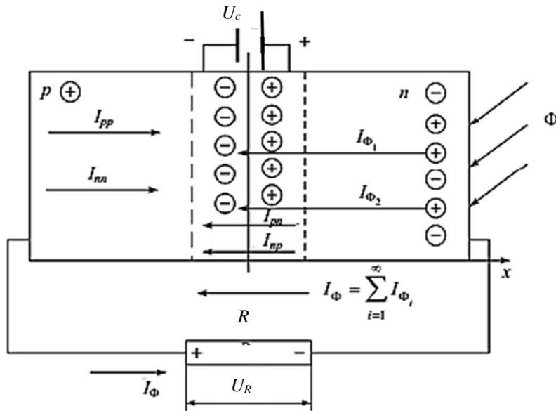
Figure 6.5 – Photovoltaic mode of photodiode operation. [12]
