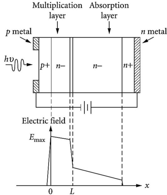
Figure 6.13 — Schematic diagram of an avalanche photodiode [1]
