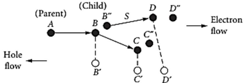
Figure 6.12 — Impact ionization process
