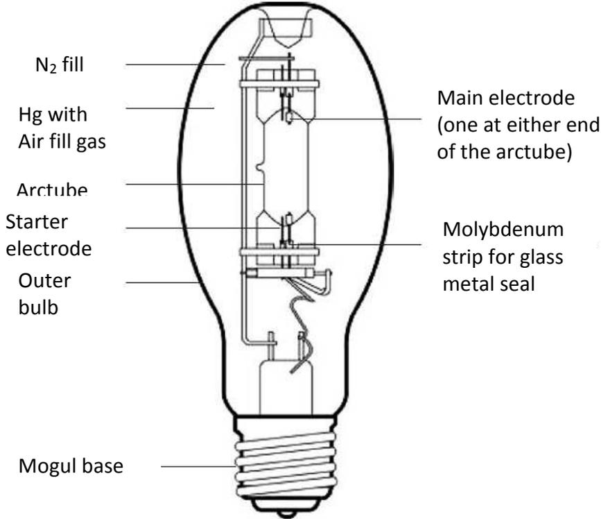
Figure4.5 – Mercury lamp construction
