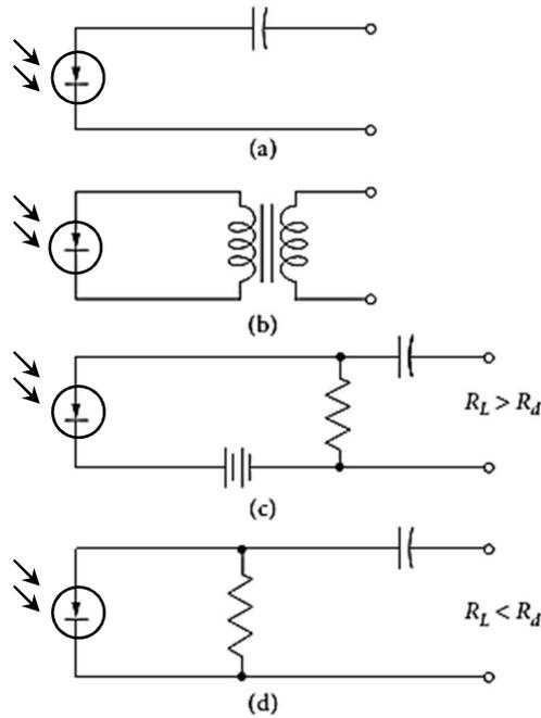
Figure 6.8 — Recommended circuits for InAs detectors: a) open circuit, b) transformer, c) reversed bias, d) fast response [1]
