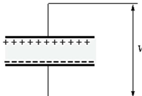
Figure 7.2 – The pyroelectric effect produces a surface charge when the temperature changes
