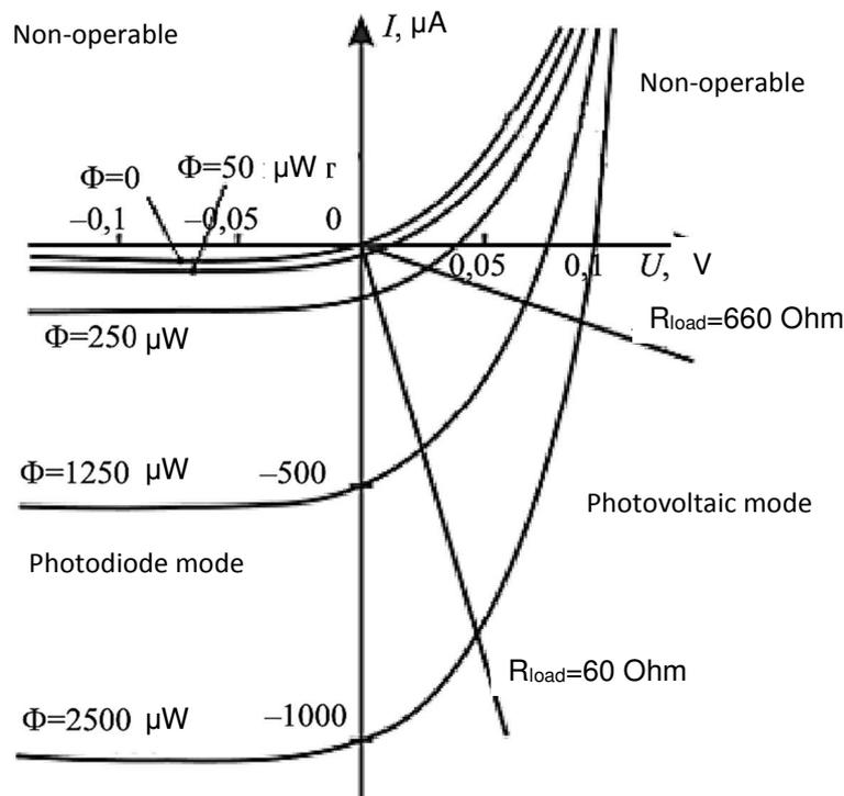
Figure 6.9 — Current-voltage characteristic of a photodiode
