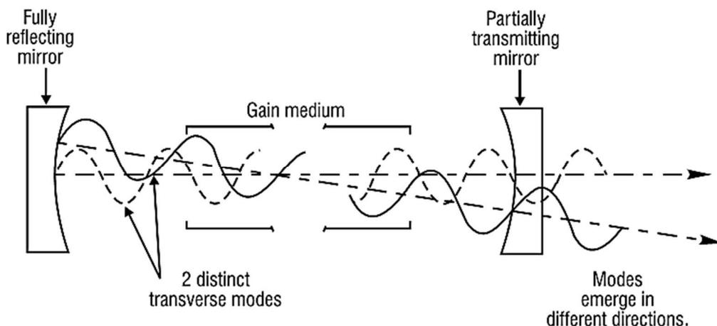
Figure 4.12 – Two transverse modes occurring simultaneously within a laser cavity. The on-axis mode is the  $TEM_{00}$  mode.
