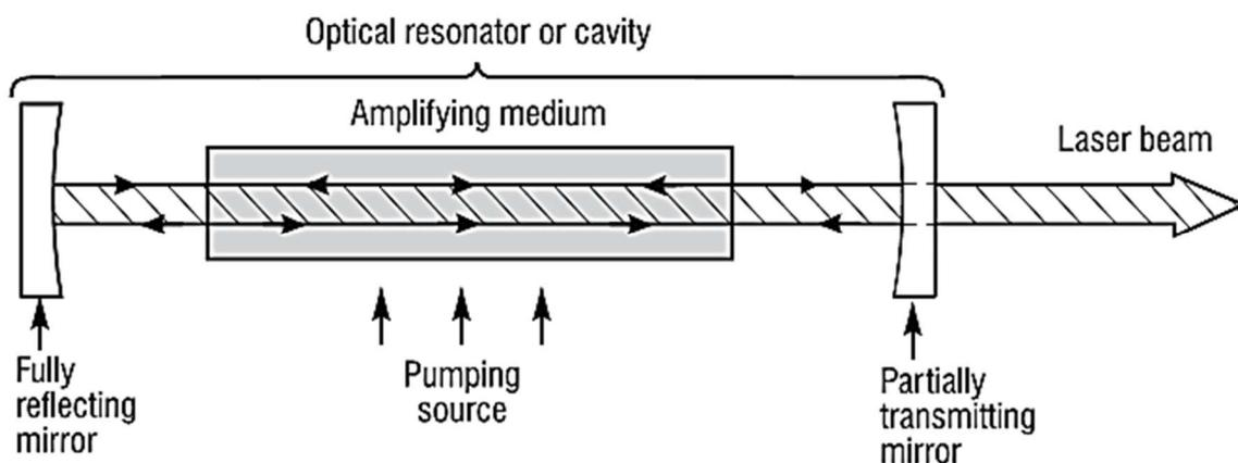
Figure 4.8 – Basic laser components including gain medium, pumping source, and mirror cavity
