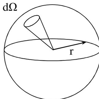
Figure 2.1 –The solid angle at the center of the sphere is the surface area enclosed in the base of the cone divided by the square of the sphere radius
