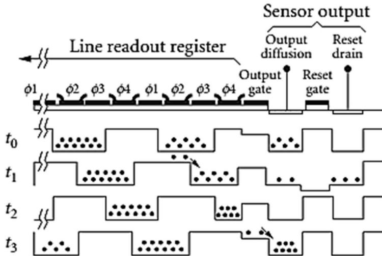
Figure 8.2 – Transmission of charge packets in a CCD line
