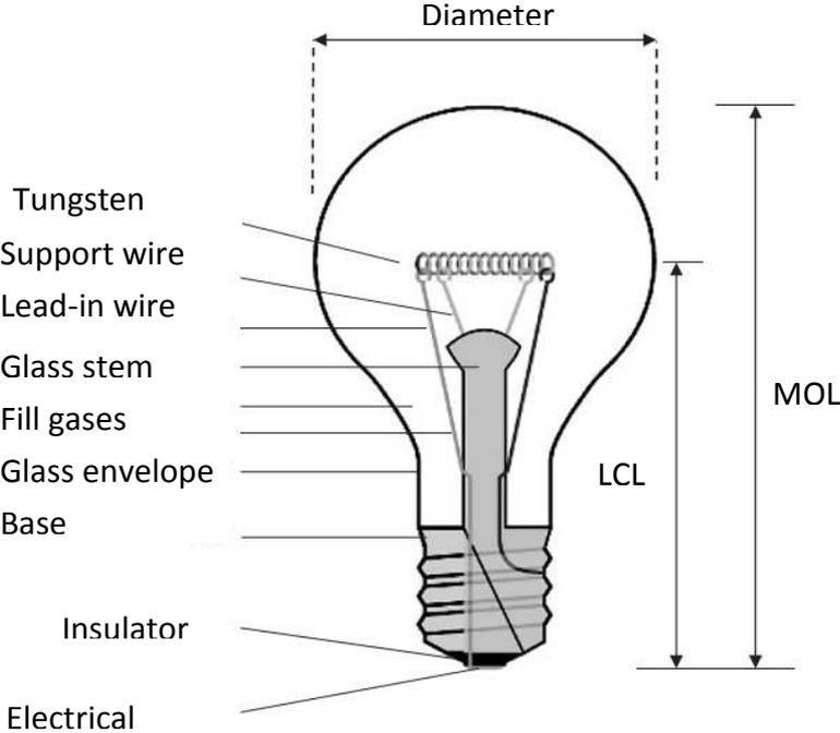
Figure 4.3 – An incandescent bulb (MOL – maximum overall length, LCL – light center length)
