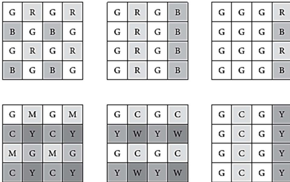
Figure 8.7— Common color filter patterns where, R=Red, G=Green, B=Blue, Y=Yellow, M=Magenta, C=Cyan, and W=White [1]
