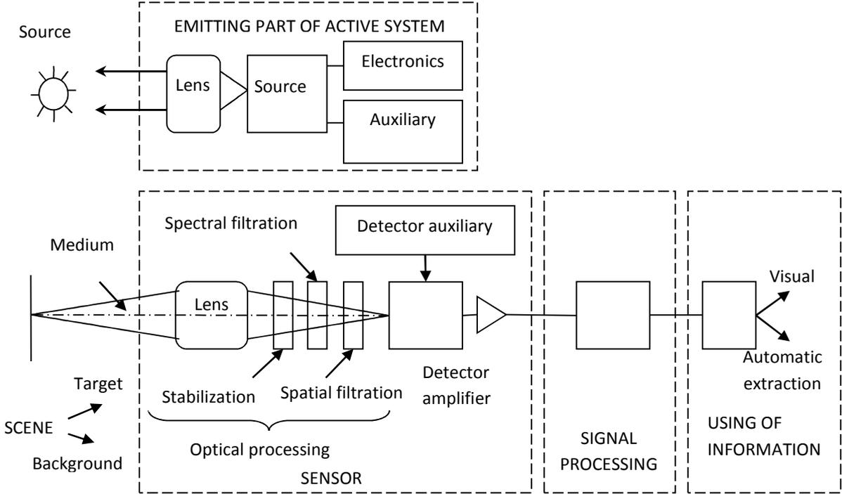
Figure 1.1 – A common layout of an optical-electronic device [2]
