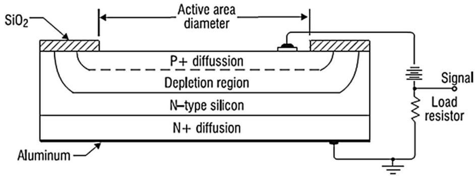
Figure 6.7 — Typical structure of a photodiode [11]
