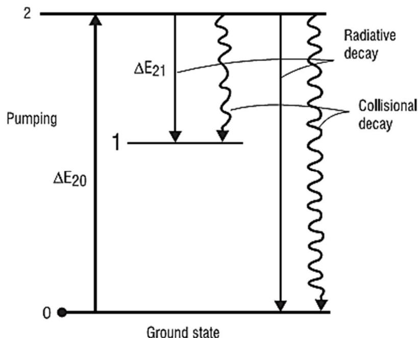
Figure 4.9 – Simplified energy diagram of an atom showing excitation and emission processes
