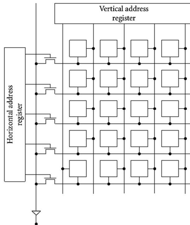
Figure 8.4 — Architectures for linear image sensors MOS photodiode array, consisting of vertical and horizontal address registers and readout line
