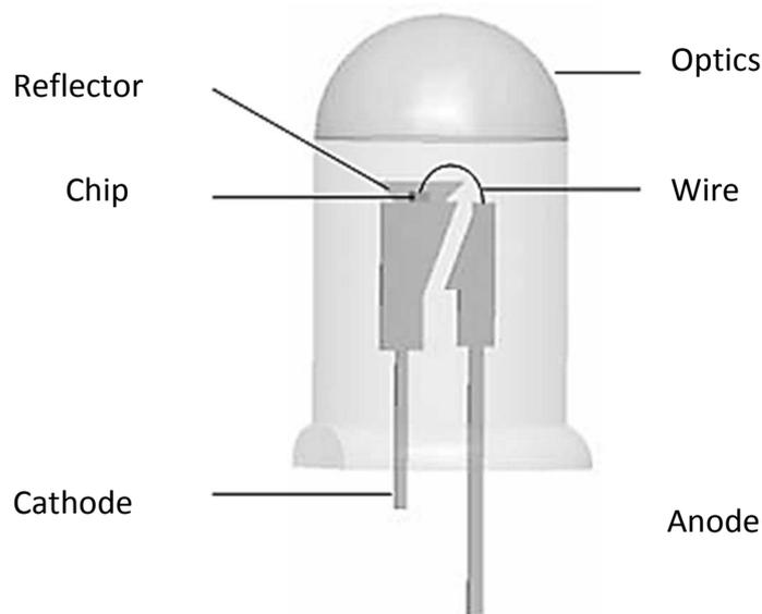
Figure4.6 – Structure of a simple packaged LED
