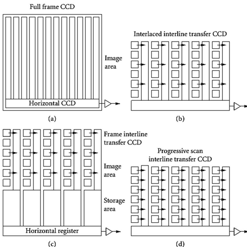
Figure 8.5 — (a) Architecture of full-frame CCD; (b) architecture of interlaced interline transfer CCD; (c) architecture of frame interline transfer CCD, in which a storage area is provided to reduce smear during readout; and (d) progressive scan interline transfer CCD, in which every photodiode is read out into the vertical CCD simultaneously
