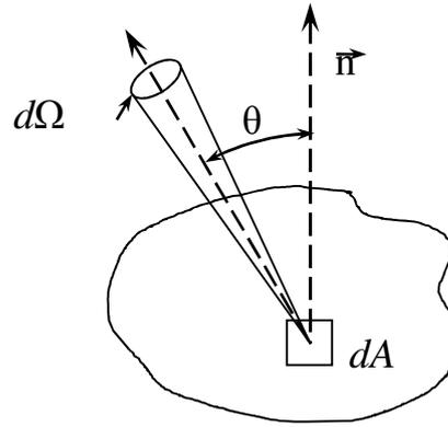
Figure 2.3 – The radiant flux emitted by the infinitesimal area  $dA$  within the solid angle  $d\Omega$ , the direction of the flux having the angle  $\theta$  to the normal to the surface element
