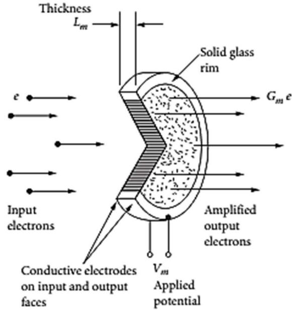
Figure 6.15 – Microchannel plate structure [1]
