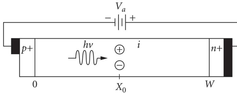
Figure 6.10 — p-i-n photodiode structure [1]
