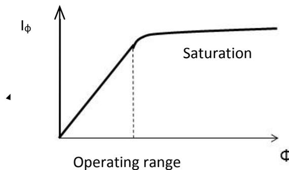
Figure 5.5 – Detector operating range
