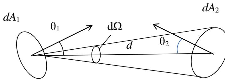
Figure 2.2 –Parameters to characterize the geometrical étendue
