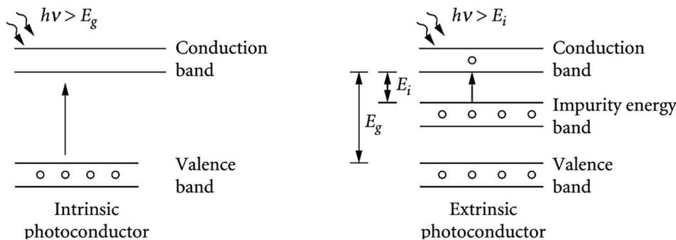
Figure 6.1 – Functional diagram of an intrinsic and extrinsic photodetector [1]
