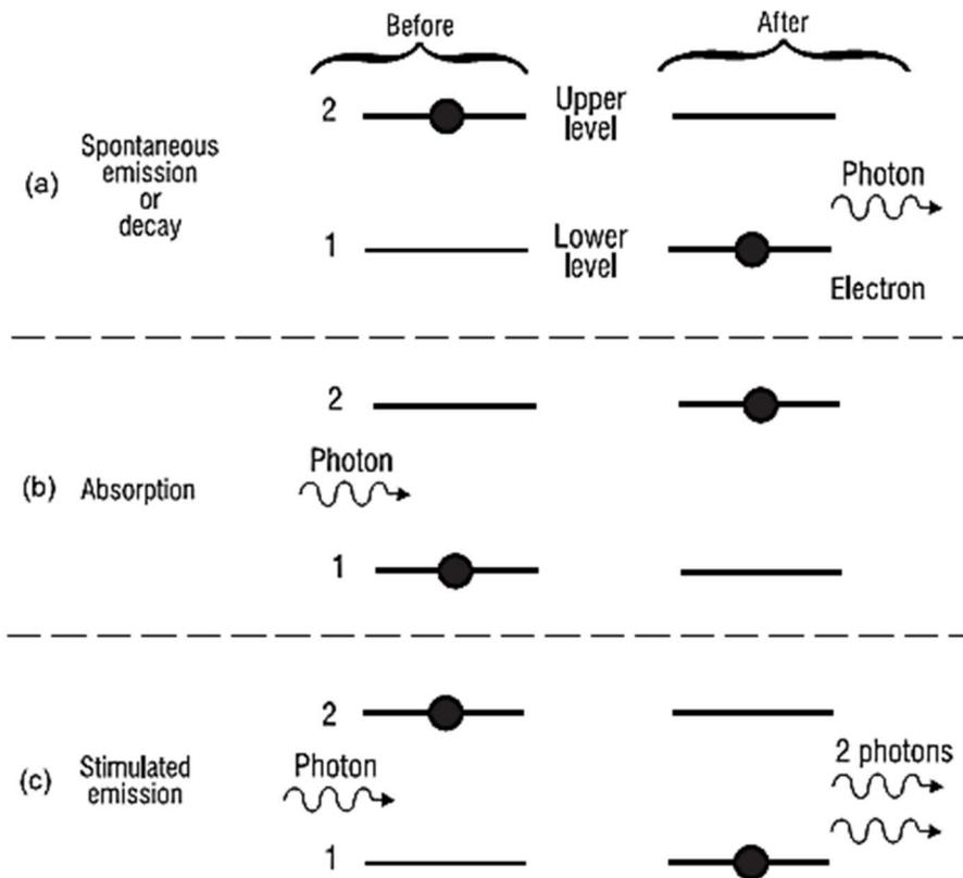
Figure 4.10 – The three radiation processes that can occur when light interacts with matter (atoms)
