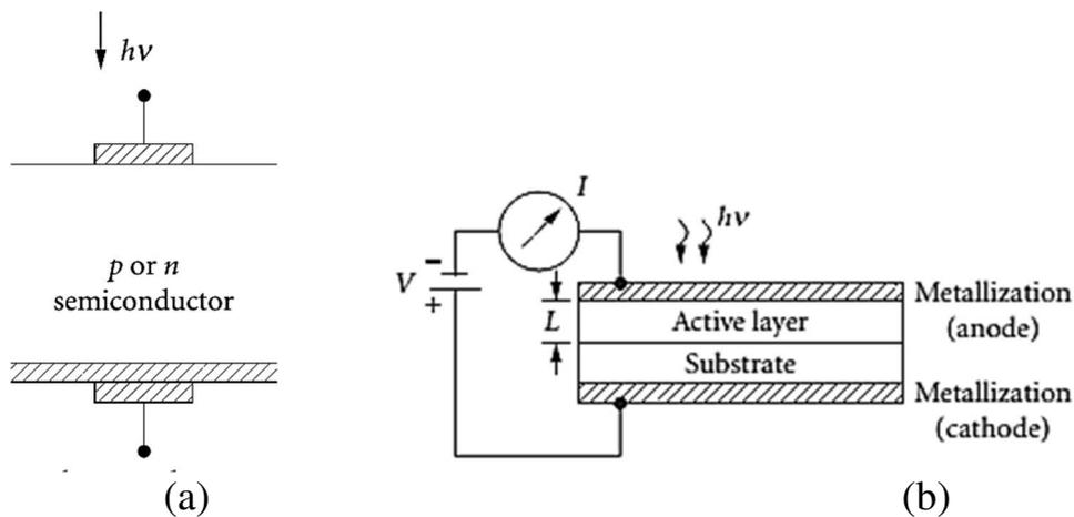
Figure 6.2 — Photoconductor structure (a) and circuit (b)
