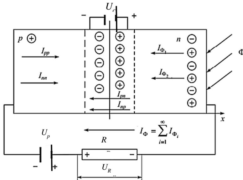
Figure 6.6 – Photodiode mode principle [12]
