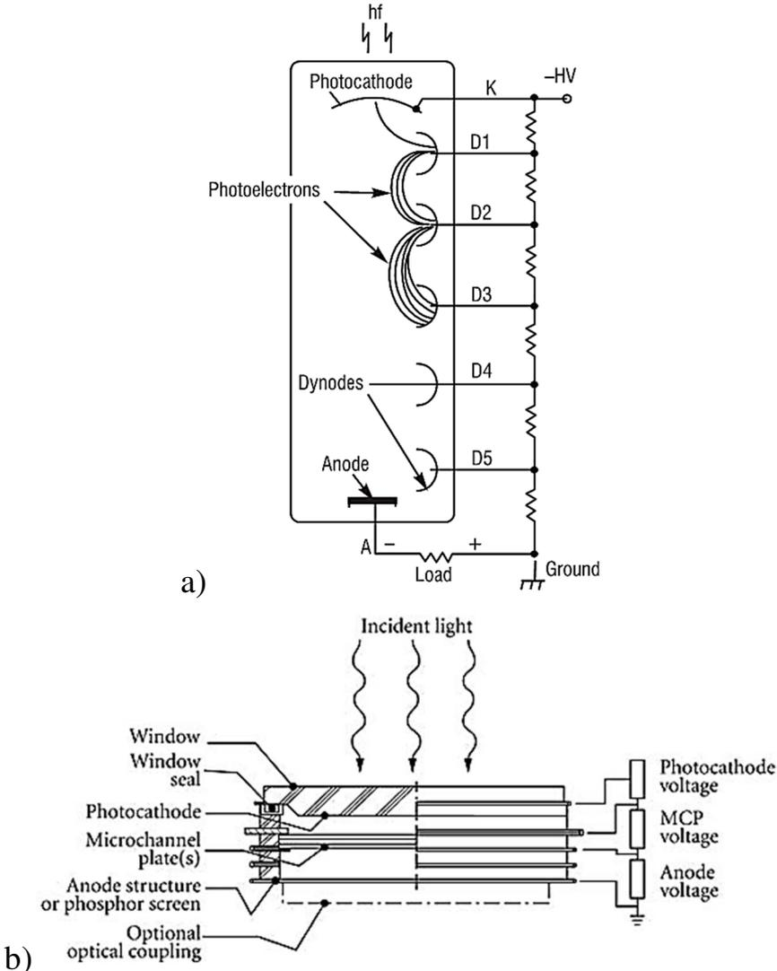
Figure 6.14 – Comparison of photomultiplier (PM) tube (a) and microchannel plate (MCP) tube (b) construction [1]
