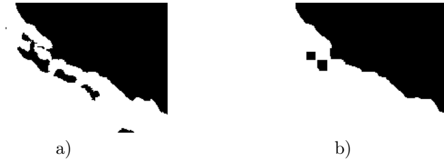
Figure 1.9. a) Result image after applying bwareaopen() function; b) result image after applying imclose() function
