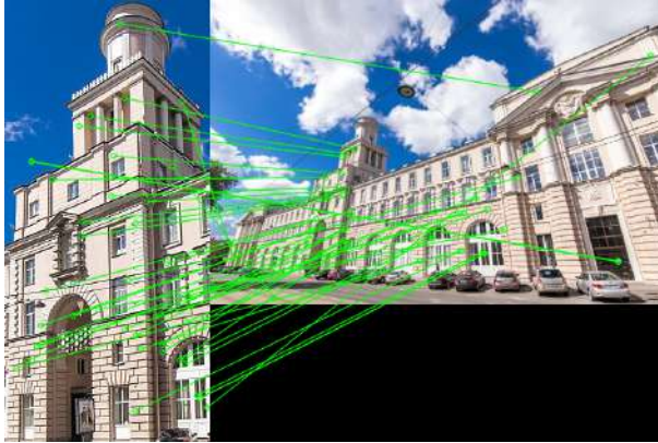
Figure 3.20. All matches with brute force method, k -nearest ratio filter and SIFT descriptors
