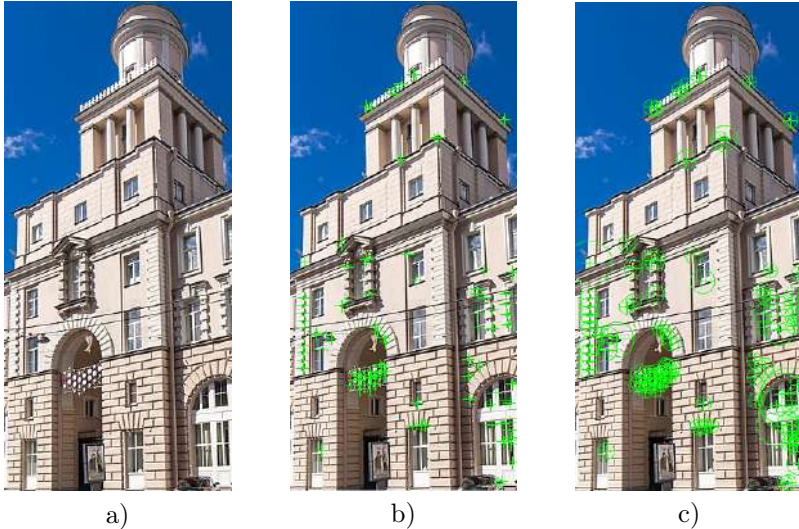
Figure 3.8. SIFT feature detector with MATLAB: a) Source image, b) 100 strongest SIFT feature points, c) 100 strongest SIFT feature points with the scale and orientation
